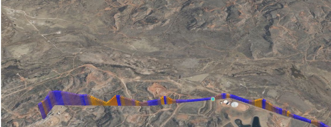
Figure 9 Elevation profiles help analysts understand patterns of internal corrosion in their pipelines.
